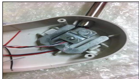
Fig 8: Typical 3 Wire Strain Gauge
